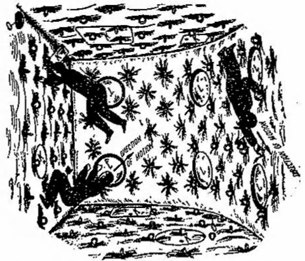
Fig. 1—A room in the observatory in space, in which weightlessness prevails and which is equipped accordingly. The walls are completely padded and provided with hand-holds. No loose object is present. K—Boxes with fastenings for keeping utensils, etc. L—Windows to admit the light. O—Openings for the conduction of air. Z—Motion by pulling along. A—Motion by pushing off.
